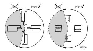
Fig. 8. Mounting for IP54.
