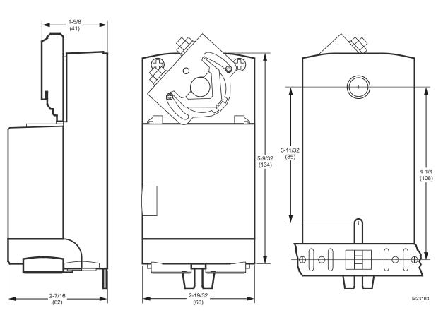
Fig. 14. Dimensions in Inches (mm).
